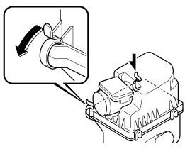
3. Lift off the air filter cover and remove the filter.
