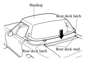
6. Slide the hardtop forward while pressing down on the rear deck latches to lock the latches, and then verify that they are secure by attempting to lift the rear of the hardtop.
