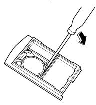
4. Put in the new battery (CR1620 or equivalent) with the positive pole (+ ) facing down.
