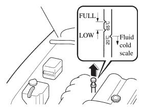
The proper fluid level is marked on the dipstick as follows.
