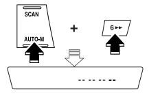
4. While the bars are displayed, input your personal code number by pressing channel preset buttons 1, 2, 3, and 4.
