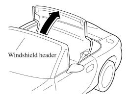
7. Fold back the front and carefully lower it to the storage area, then put the latches in the locked position.
