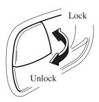
To lock any door with the door-lock knob from the outside, push the door-lock knob to the lock position and close the door. This does not operate the other door locks.
