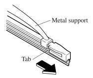
3. Remove the metal stiffeners from the blade rubber and install them in new blades.
