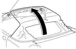
8. After securely hooking the top latches onto the windshield header, push each latch up with the palm of your hand until the lock buttons click and the latches are locked.
