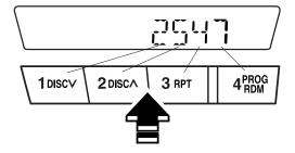
5. While the code number is displayed, press the auto memory button (AUTO-M) and the channel preset button 6 simultaneously for about 2 seconds and "CODE" appears.
