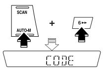
3. Again press the auto memory button (AUTO-M) and the channel preset button 6 simultaneously while "CODE" is displayed (within 10 seconds). The display will exhibit bars.
