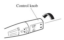
Accelerate to the desired speed. Turn the control knob to SET/COAST and release it immediately.
