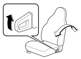
Make sure the lever returns to its original position and the seatback is locked in place by attempting to push it forward and backward.
