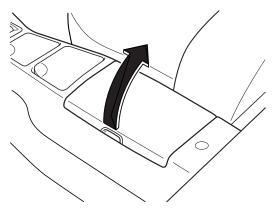
To open the fuel-filler lid, pull up on the remote fuel-filler lid release.
