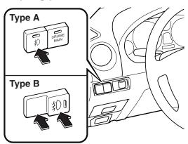
To turn on the fog lights, first turn the headlight switch to the <sup></sup>□□□ position. Then press the fog light switch. To turn the fog lights off:
