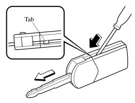
2. Insert a small screwdriver into the slot and gently pry open the transmitter.
